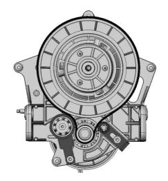
Old brush drive with one tension roller and a short drive belt
