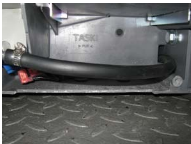
New hose EPDM placed in the machine
