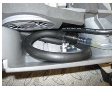
New hose EPDM placed in the machine
