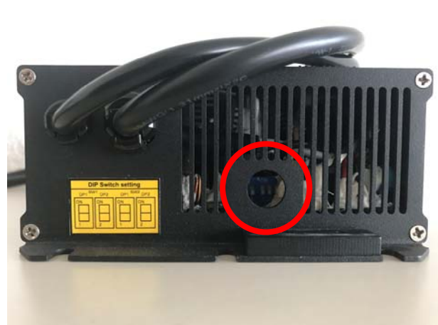
DIP switch access
