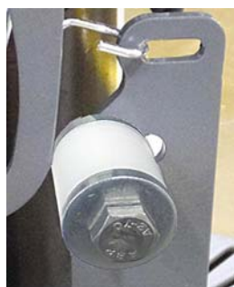
New kit slide roller assembly (Disk/Orbital models)
