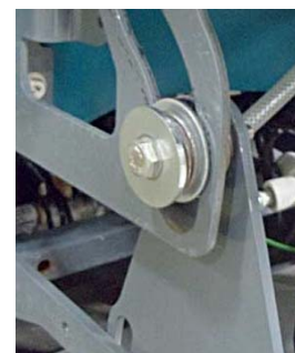
New kit slide roller assembly (Cylindrical models)
