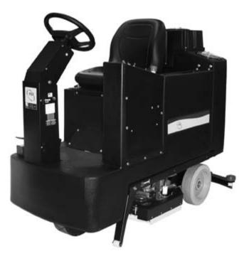
The Champ series scrubbers from NSS® are the ride-ons with big ride-on power. Their 36V electrical system package delivers up to 30 percent more run time than a comparably configured 24V machine, so the Champs give you more of what you expect from a ride-on autoscrubber.
