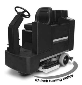
The single front-drive wheel pivots 90 degrees in both directions; most other machines do not. The Champ 2929 turns around in 67-in. of space, the 3529 in 70-in. This means the Champ scrubbers can turn around comfortably in a 6-foot wide aisle.
