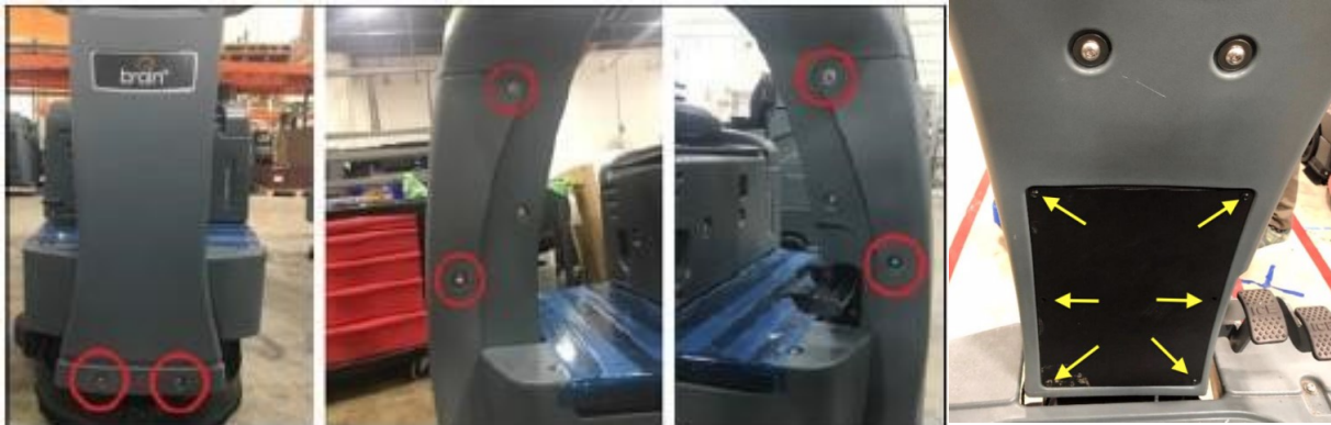
Removing both access panels
