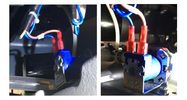
The wire(s) should **not** be broken, frayed, loose or disconnected from the Solenoid, as shown below.
