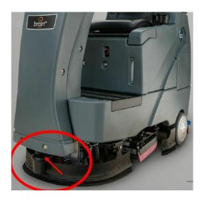
The following show the kind of photos which help diagnose potential LIDAR damage.
