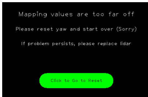
Figure 21 Lower LIDAR yaw calibration error – reset and train routes again
