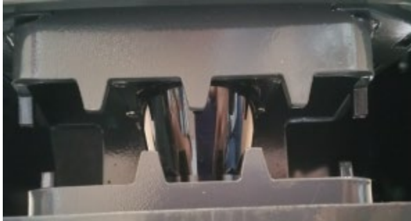
Figure 11 Lower LIDAR flush with lower LIDAR protector
