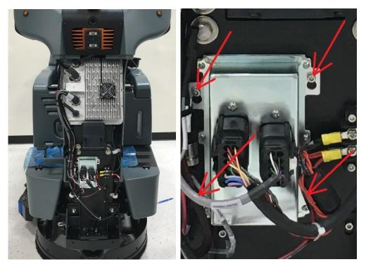
Loosen the four 3 mm hex screws above the eyelets, decouple the two black plugs and remove the Motor Amplifier
