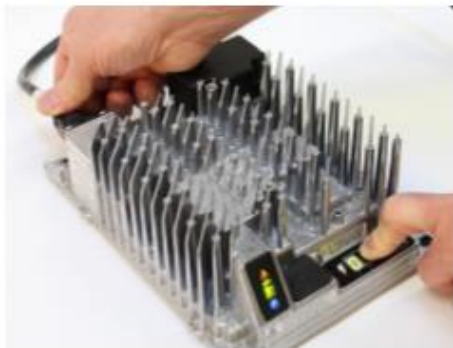
Figure 2: Reconnect AC input while holding the Select Charge Profile Button.
