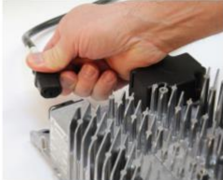
Figure 1: Disconnect AC input from the charger.
