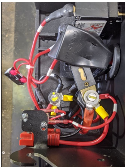
Figure 15: Install the new charging connector
