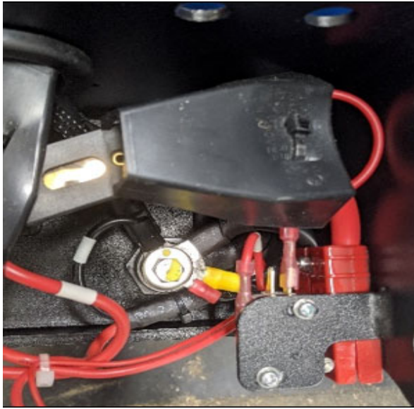
Figure 8: Remove the terminal cover
