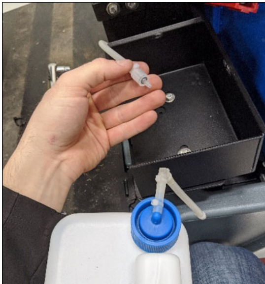
Figure 5: Disconnect and remove the detergent tank
