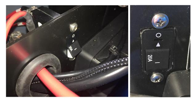
Key-off, trip and reset the BCM circuit breaker by pushing the end of a paperclip in the slot above (O)FF. Once it pops out, push it back in.
