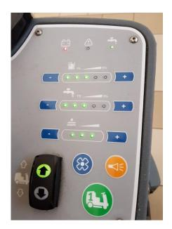
Key-off and do a hard reboot by unplugging the red battery coupling for 2 minutes.
