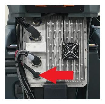
Reconnect batteries to test for voltage
