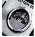
To observe this reading - turn on the master switch, observe the meter, turn off the master switch.
