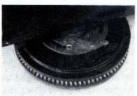
Remove the center cutout of the 14" pad (W27) or the 17" pad (W33).
