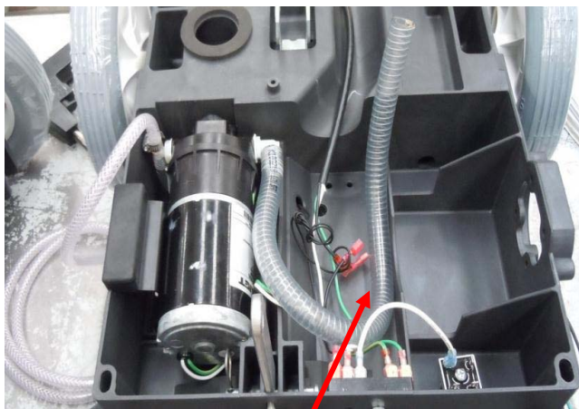
Fig 4 - Incorrect Hose Routing
