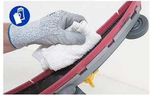
**3.** Rotate squeegee blades when wiping edge becomes worn (rounded). Each blade has four wiping edges.
