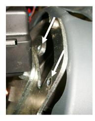
Step #9: Completely remove the spring from the frame and tensioner arm.
