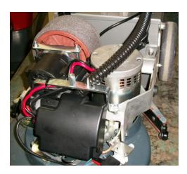
Step #5: Remove the solution tank and expose the main components.
