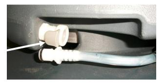
Step #4: Depress gray button and unplug the solution line from the solution tank.
