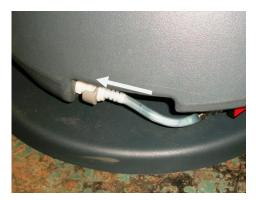
Step #17: Reinstall the solution tank and the solution line. Note: The solution line is installed by pressing the hose into the QD fitting. You will hear a "click" when properly installed.
