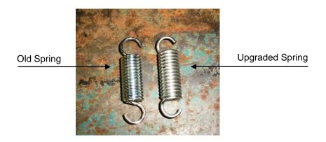
**Step #10:** Locate the upgraded spring. **Note:** *The new spring's hooks face the same direction, whereas the old spring's hooks are opposite of one another.*
