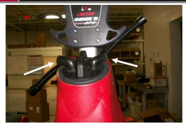
**Step #18:** Reinstall the recovery tank along with the vacuum hoses.
