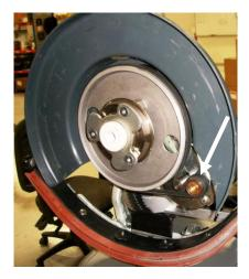
Step #7: Tilt the machine back (with the squeegee in the up position) and remove the belt.
