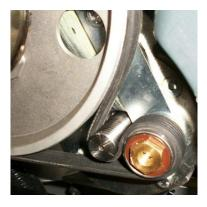
Note: To remove the belt, slip it off the main pulley and out of the tensioner assembly.
