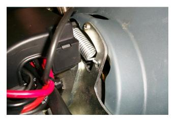
Step #11: Using needle nose pliers, hook one end of the spring into the frame.
