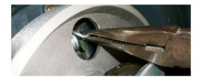
**Step #12:** Turn the pulley until the tensioner arm is visible from the bottom of the machine. Next, use needle nose pliers and hook the spring as shown above.
