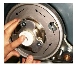
Step #15: Continue installing the belt by rotating the brush drive hub in a counter-clockwise motion. Note: This will insure the belt is aligned properly with the other pulleys.
