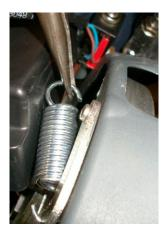
Step #8: Using needle nose pliers, unhook the spring from the tensioner as shown above.
