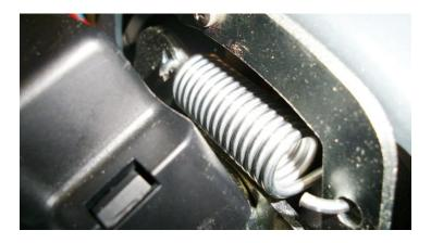
**Step #13:** Upon installation of the tensioner spring, the assembly should look like the picture above.
