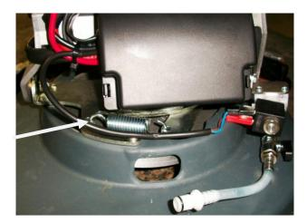
Step #6: Locate the belt tensioner spring (E81530) in the front of the machine.
