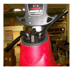
Step #1: Remove the vacuum hoses that are attached to the recovery tank lid.
