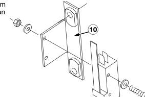
4. Mount the new switch bracket (10), squeegee pivot plate (14), and catch bracket (7) with hex screw (13), and mounting hardware from the old housing. Secure the side of the squeegee pivot plate (14) with the two rivets (15).
