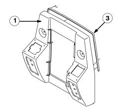
2. Install the new housing on the machine. Connect the lanyard strap to the new housing (1). Leave the new housing (1) tilted open to access the wire harness connections for instruments.
