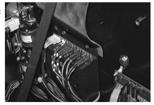
5. Unplug the potentiometer from the controller. Unplug the wire harness from the stop switch. Loosen the speed control handle latch, and remove the shroud locking bracket from behind the shroud. Set the locking bracket aside. Slide the adjustable steering housing out of the slots in the fixed steering housing. (Refer to FIG. 1)
