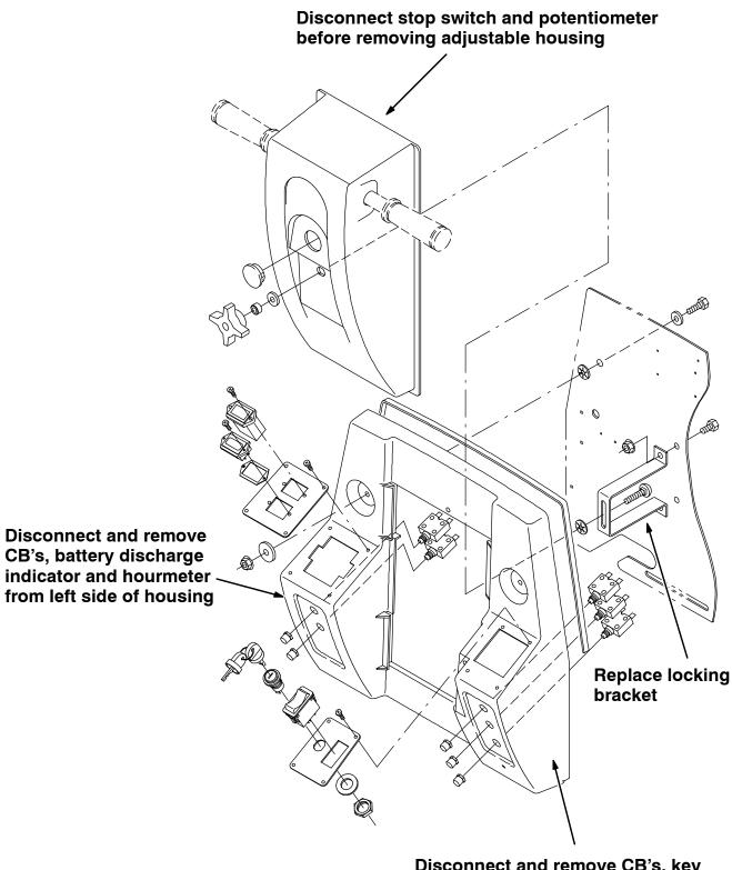
Disconnect and remove CB's, key switch and scrub switch from right side of housing
